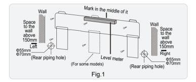
(2) Drill a piping hole with the diameter of  $\Phi$ 55mm or  $\Phi$ 70mm on the selected outlet pipe position. In order to drain smoothly, slant the piping hole on the wall slightly downward to the outdoor side with the gradient of 5-10°.(As show in Fig.2)
