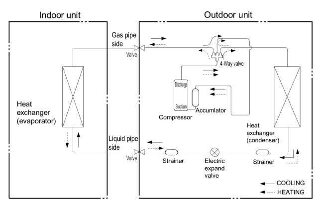
Connection pipe specification: Liquid pipe:1/4" Gas pipe:3/8" 12K Gas pipe:1/2" 24/28K
